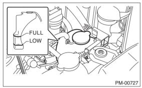
3) Remove the radiator cap and make sure that the radiator is filled with engine coolant up to the filler neck position.
